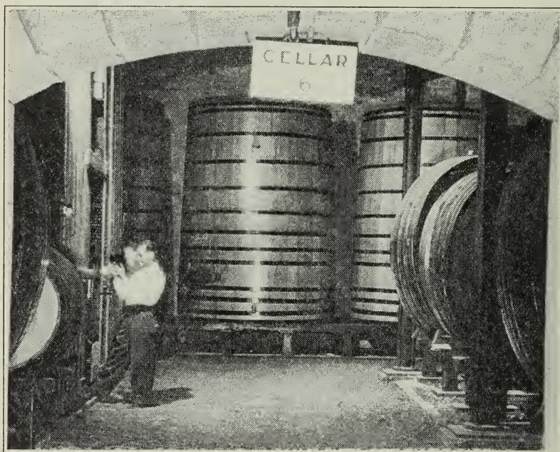
Fig. 10.—Storage containers: oak tanks in the background, ovals and puncheons in the foreground.
